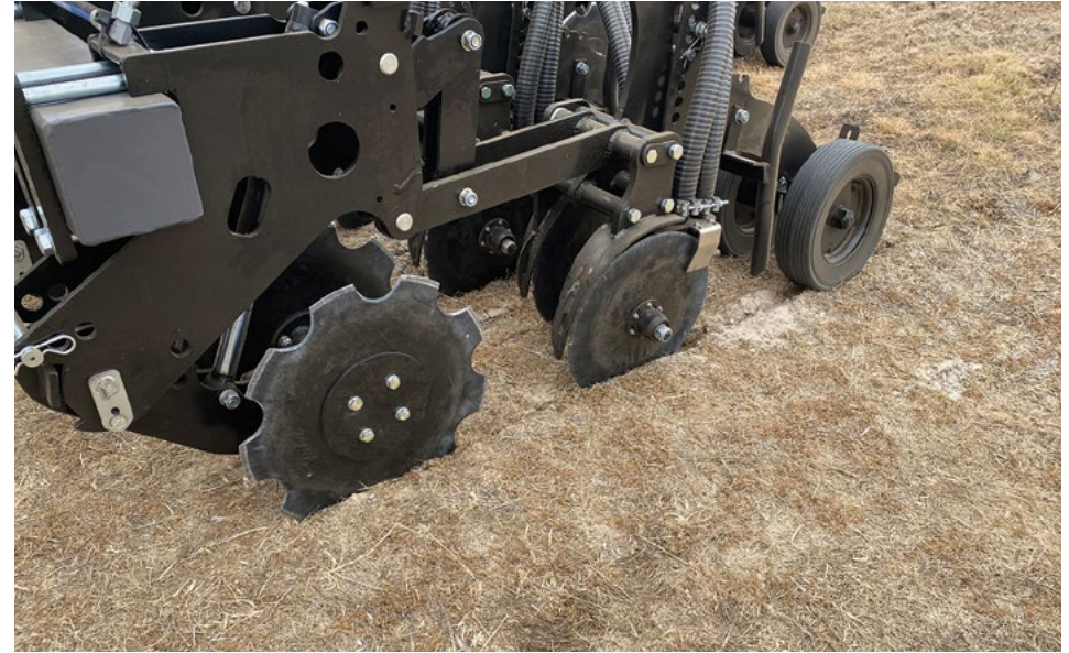
CUTTING COULTER SLICE EASILY THROUGH THE SOIL, ALLOWING FOR ACCURATE SEED PLACEMENT
