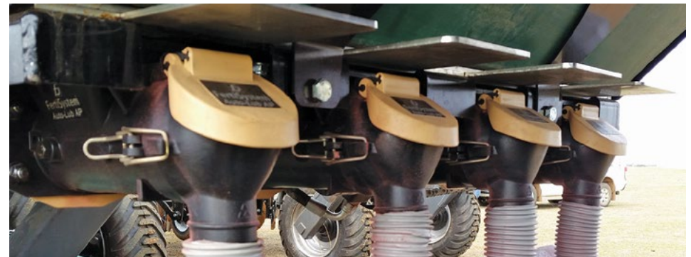
THE FERTI-SYSTEM IS OPTIONAL - OTHERWISE STANDARD PIKET SEED METERING UNITS WILL BE USED
