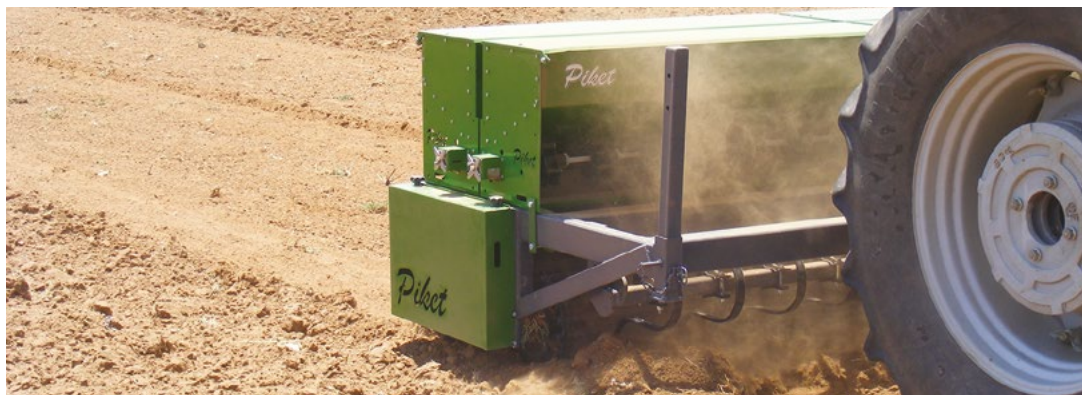
SEEDS ARE COVERED WITH A THIN LAYER OF SOIL DURING THE COMPACTION PROCESS
