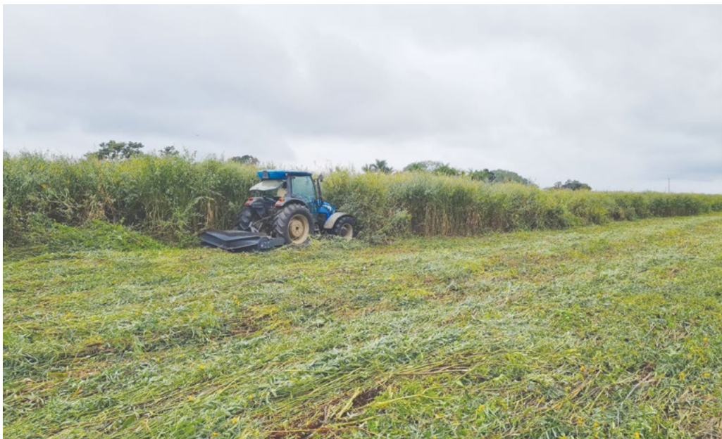
CRIMPS THE STALKS WITHOUT CUTTING IT, REDUCING THE POSSIBILITY OF RE-GROWTH
