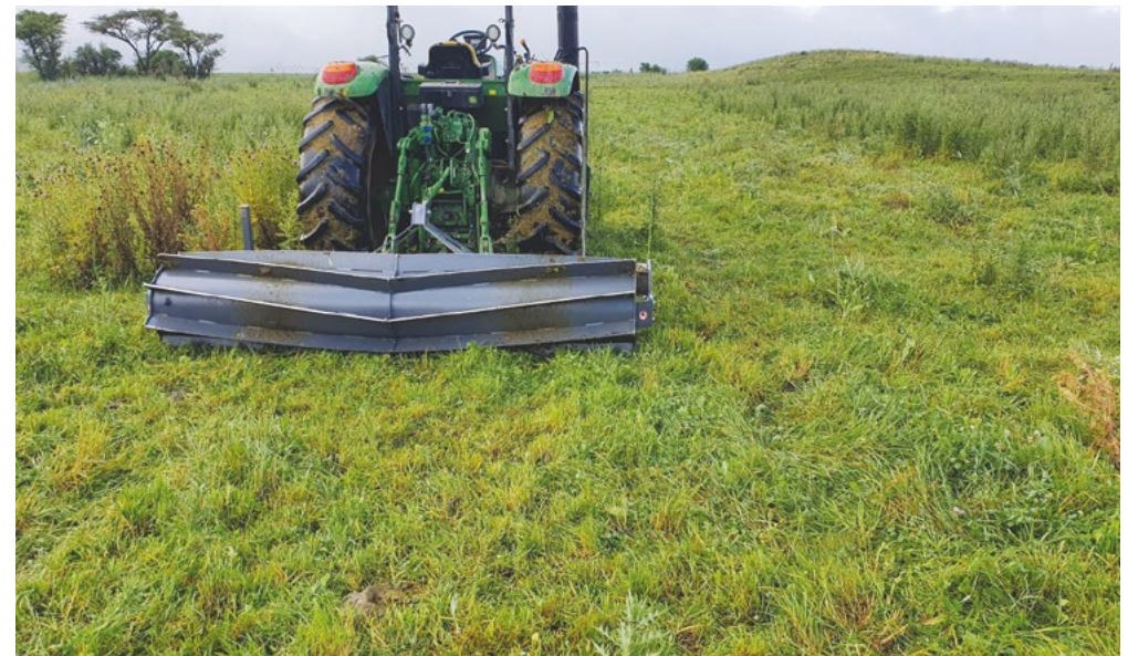
BLADE PROFILE ENSURES SMOOTH ROLLING ACTION & MAXIMUM DOWN FORCE PER BLADE
